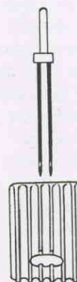
Fig. 8-15. Twin needle and the bottom of the 5-grooved pin-tuck foot it matches. Placing the grooves over previously sewn tucks regulates the distance between tucks.
