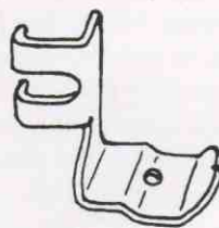
Fig. 1-7. The gathering foot is as easy to use as a regular presser foot. The longest stitch length combined with tightened upper tension produces the fullest gathers.
