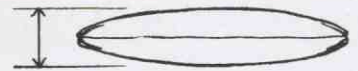
Fig. 11-46. Little pillow profile. To estimate height, choose a realistic measurement for the imagined depth that stuffing will produce when inserted into the casing.
