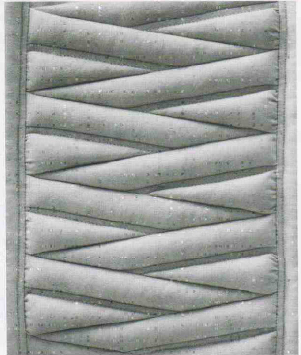
XI-17—Topstitched channels separate most of the half-rounds in a design that zigzags between half-round borders at the sides.
