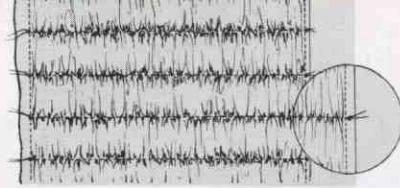
Fig. 2-2. On the left, gathered stitching that stops at the fabric's edge secured with bobbin-and-needle-thread knots and a vertical line of machine stitching that crosses each knot. On the right, gathered stitching that stops within the fabric secured with bobbin-and-needle-thread knots and a vertical pin tuck that catches each knot inside the tuck seam.
